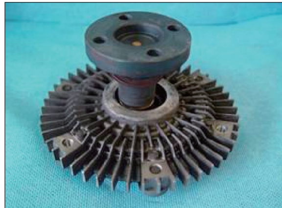
Fan clutch bearing blocked → breakage
