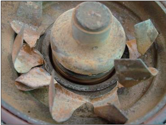
Impeller Corrosion
